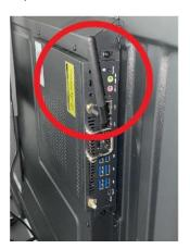
**Caution**: Do not install the OPS Module while the interactive panel is powered on. This may damage the device. Always install the OPS while the panel is powered off.
