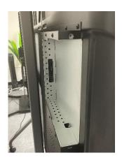
2. Insert the OPS Module into the slot. Make sure the power button is on the bottom. Also, install the two screws removed in step 1 to secure the OPS Module.
